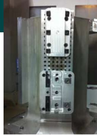
Fixtures mounted on company's Mori-Seiki Tombstone
