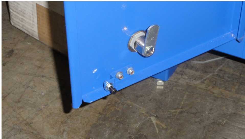
Location of safety switch screw on bottom inside of left door.
